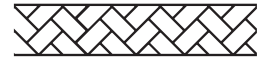
HERRINGBONE HEADER BRICK SIZE: 3\frac{3}{8}'' \times 7\frac{3}{16}'' ROLL WIDTH: 8\frac{9}{16}'' JOINT WIDTH: \frac{1}{2}''
