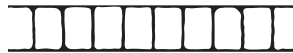
COBBLE HEADER BRICK SIZE: 4\frac{3}{8}'' \times 7\frac{1}{2}'' ROLL WIDTH: 8\frac{3}{8}'' JOINT WIDTH: \frac{1}{2}''
