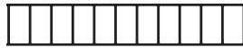
BRICK HEADER BRICK SIZE: 3\frac{1}{8}'' \times 7\frac{5}{8}'' ROLL WIDTH: 8\frac{3}{4}'' JOINT WIDTH: \frac{1}{2}''
