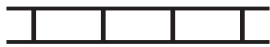
EDGE BRICK HEADER BRICK SIZE: 4\frac{1}{8}'' \times 8\frac{13}{16}'' ROLL WIDTH: 5\frac{1}{8}'' JOINT WIDTH: \frac{1}{2}''
